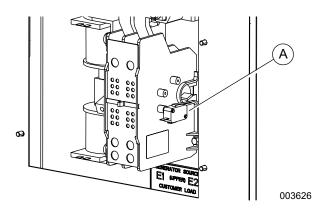
Figure 2-5. Auxiliary Contact
