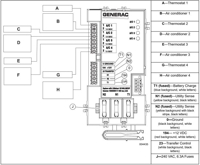
Figure 2-4. Typical SACM Connections
