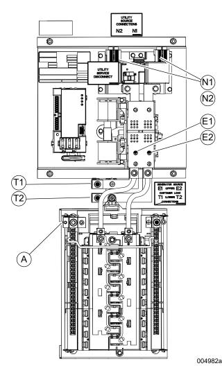
Figure 2-3. Wiring Connections
