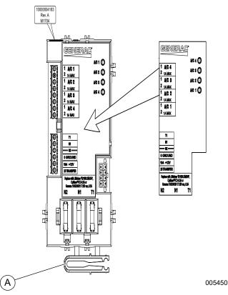
Figure 3-2. Fuse Removal and Installation Tool
