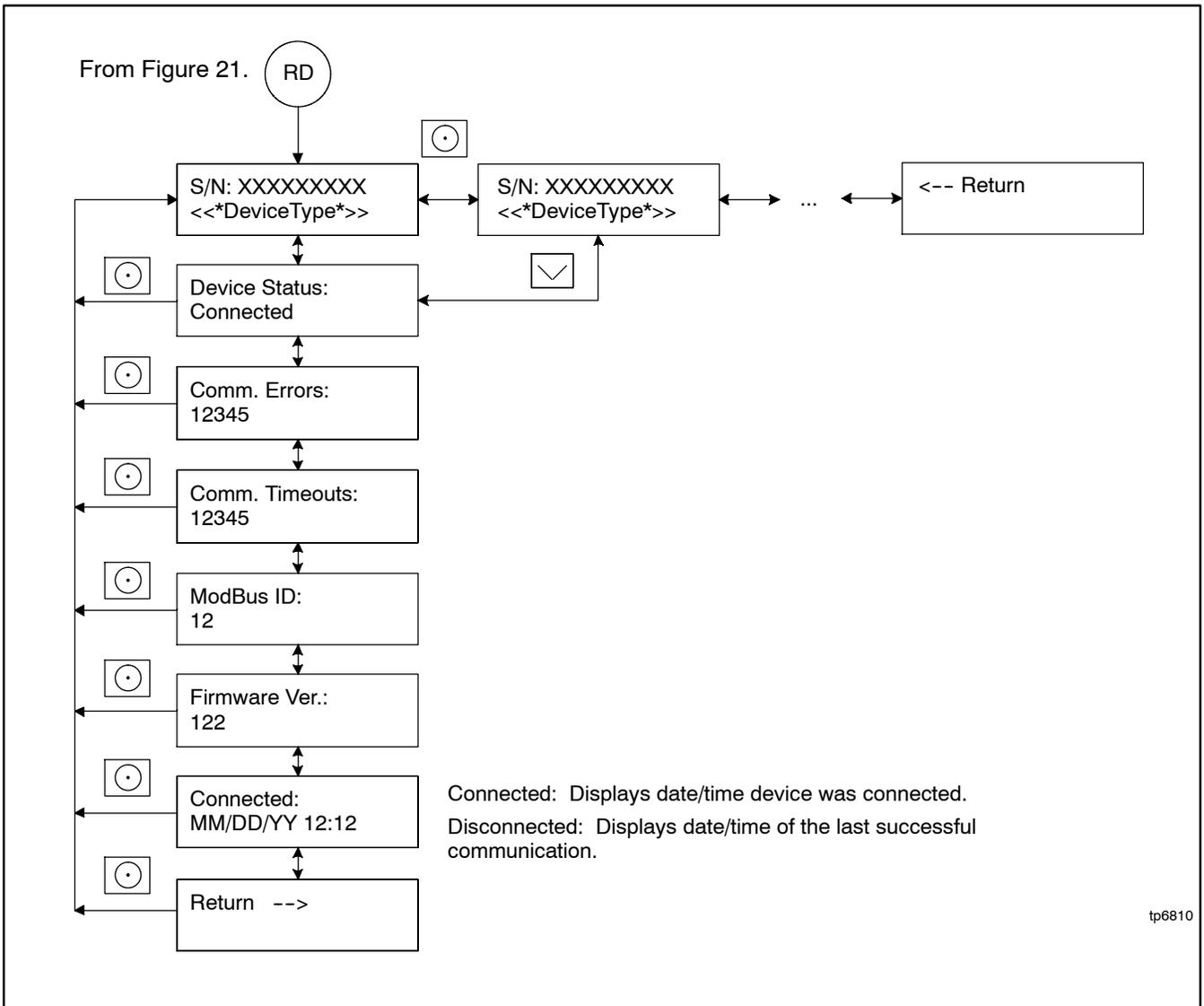
**Figure 22** RDC2 Controller, Remote Devices Submenu
