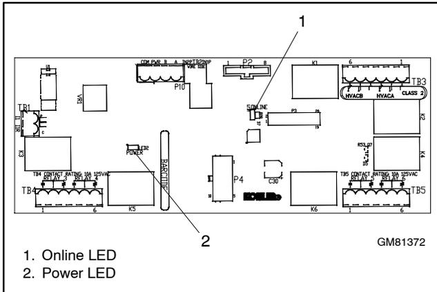
**Figure 20** LEDs on the Load Shed Circuit Board
