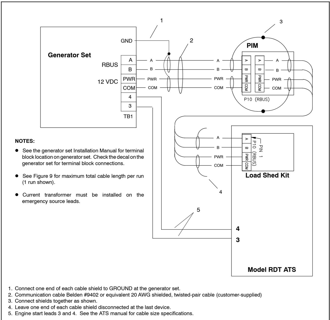
**Figure 12** Alternate RBUS Communication Connection Details with Model RDT Transfer Switch and Optional Programmable Interface Module (PIM)
