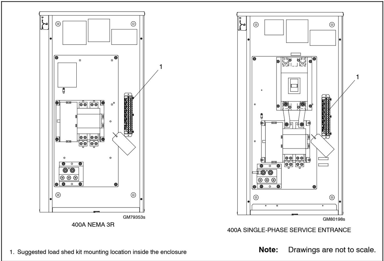
**Figure 29** Recommended Kit Mounting Locations, 400 Amp Model RXT Transfer Switches without Mounting Holes or Hardware
