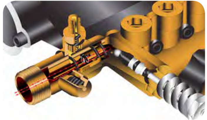
PowerBoost® Technology high pressure water flow in our C30 pump
